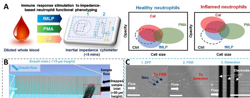
Figure 1: Impedance mapping of neutrophil immune response using inertial impedance cytometer. (A) Experimental workflow (B) Simulation showing 3D focusing at the inlet region. Red box indicates confined sample stream. (C) High speed images showing neutrophil sorting and focusing at different stages of the platform. Scale bar = 100  $\mu$ m.
