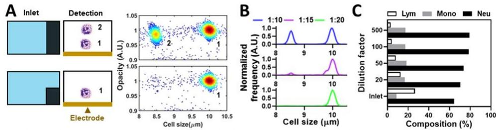
Figure 2: Platform characterization (A) 3D particle focusing at inlet and detection region for devices with and without stepped inlet. Black and blue indicate sample stream and sheath stream respectively. (left) Impedance profiling of 10  $\mu\text{m}$  beads without and with stepped inlet (right). (B) Quantification of particle equilibrium positions based on cell size at different flow rate ratios. (below) Relation between blood dilution and (C) sorted leukocyte compositions
